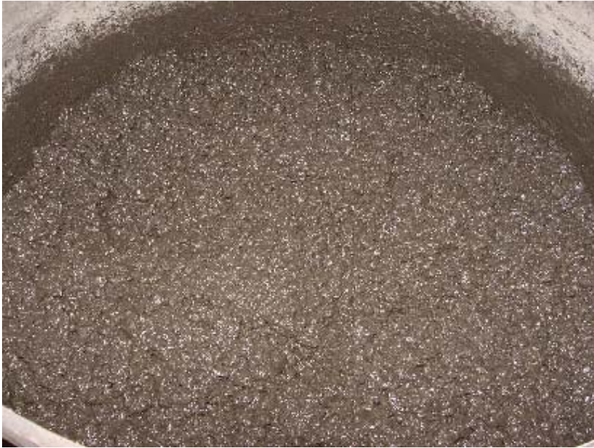
FIGURE 6: Fresh Geopolymer Concrete Ready for Placing (Hardjito and Rangan, 2005)
