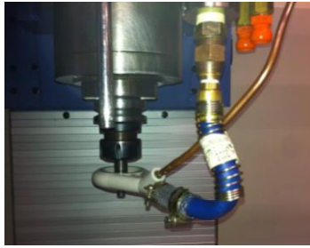
(c) Combined cold air and MQL nozzle
