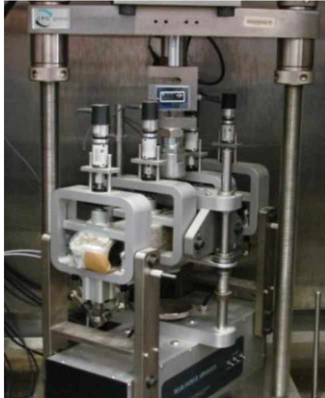
Figure 3: IPC four point Bending test rig
