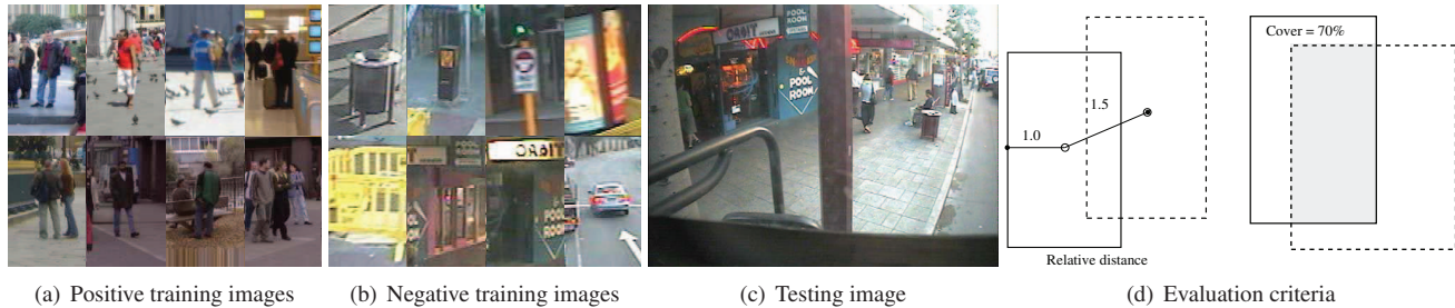
Fig. 3. (a) Examples of the INRIA dataset and (b–c) the Perth dataset that were used for training and testing in our experiments. (d) Evaluation criteria for comparing the ground truth (solid) bounding box with the detected candidate bounding box (dash).
