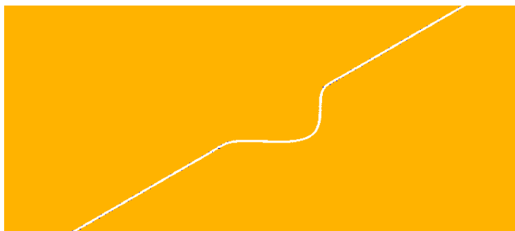
Fig. 6. First vibration mode of the outer pipe
