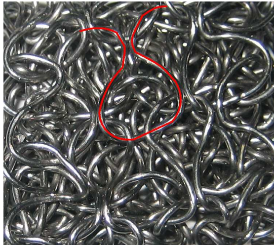
Figure 1. Image of compressed knitted metal filter showing strophoid-shaped knit loop. This particular filter would normally be used in an automotive SRS system
