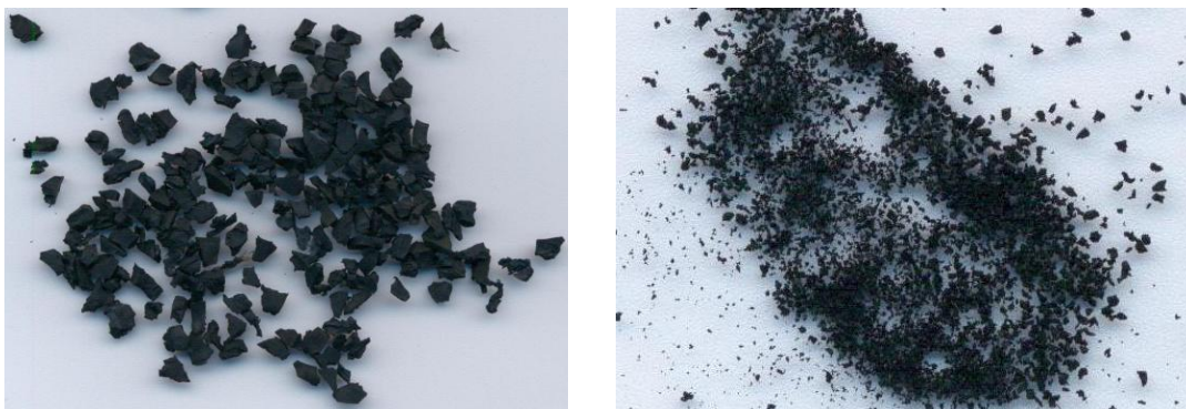
FIG. 1. Photographs showing the grain (left) and tire powder (right) used.
