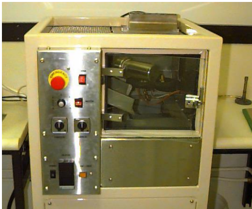
Figure 1. Gas Fired Reactor (LHS, stainless steel bomb mounted horizontally) and an example of a time - temperature profile (not indicative of actual profiles used in the present work – shows heat-up and cool down rates and temperature stability)
