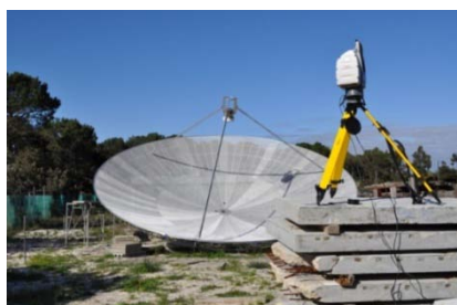
Figure 1: Satellite dish and the setup of the scanner to capture the surface.
