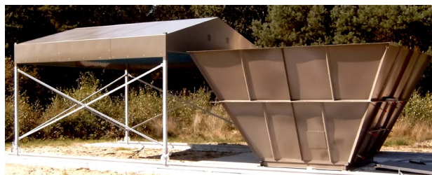
Fig. 4. A device constructed by ASTRON [15] for measuring noise from an antenna/LNA combination, which is placed at the bottom of the inverted pyramid (right). The metallic sides reflect all radiation towards the “cold” sky, which is used as a low-temperature reference. The cover (left) can be slid over the top of the device. It contains absorber at ambient temperature to act as a high temperature reference. Using these known reference radiation temperatures, noise properties of the antenna/LNA combination can be derived.
