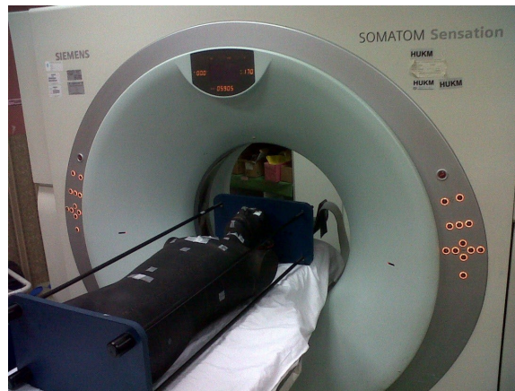
FIG. 1. Image showing that the TLDs were securely placed on the skin surface of the anthropomorphic male Alderson RANDO phantom at the targeted radiosensitive organs.
