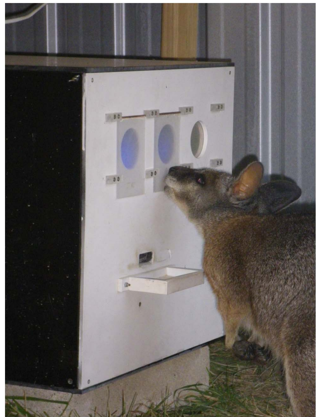
Figure 1. Wallabies readily used the automated operant conditioning setup for colour vision experiments. Light stimuli were projected onto diffuser flaps that also served as the trigger when the animal pushed to indicate a stimulus choice. If correct, a food reward was delivered into a feeder bowl under the stimuli. Photo copyright: W. Ebeling.
