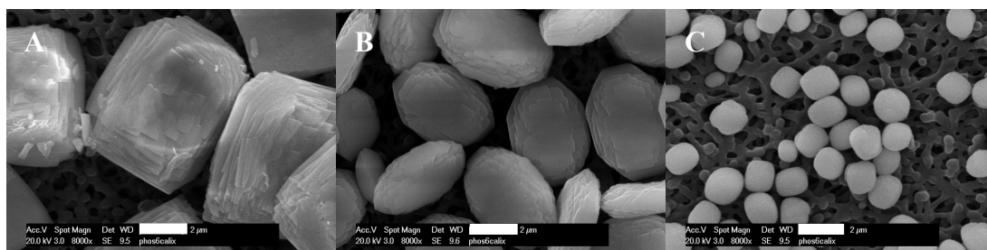
Figure 4. SEM images of barium sulfate particles formed in the presence of (A) 0.0003 mM (B) 0.006 mM and (C) 0.011 mM p -phosphonic acid calix[6]arene, 3 , (size bars are all 2 µm).
