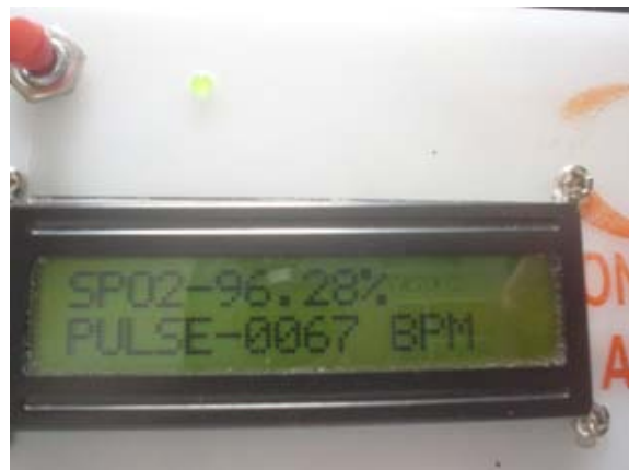
Figure 8: LCD display showing SpO 2 and Pulse Rate
