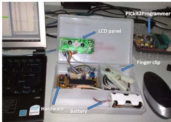
Figure 1: Experimental set-up of pulse oximeter
