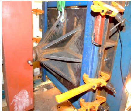
d) Impactor, strike plate, confining frame, and support frame
