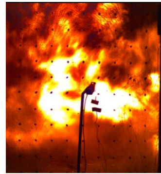
17ms back glass ply cracked
