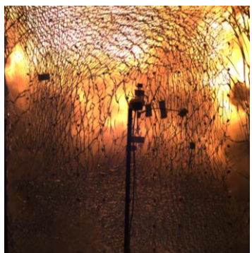
21ms glass severely damaged
