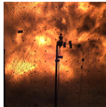
16ms back glass ply cracked
