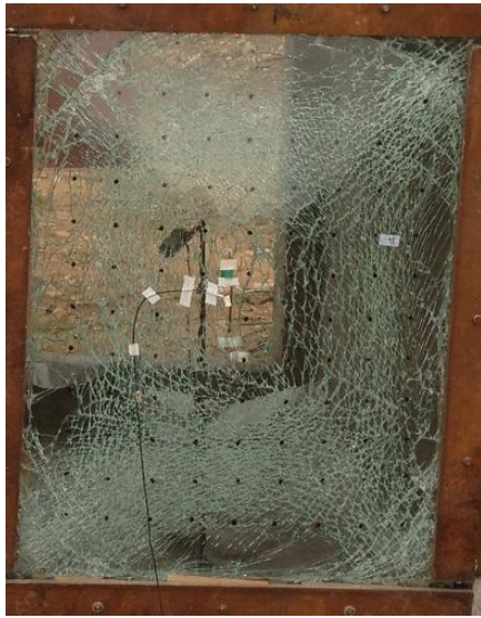
Figure 14 Pane failure patterns
