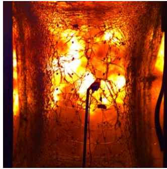
30ms pane pulled out along two vertical sides
