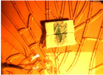
20ms outer glass ply cracked
