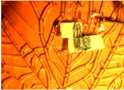
6.7ms outer glass ply cracked
