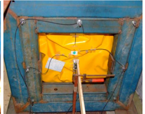
e) Laminated glass specimen setup in frame with LVDT
