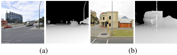
Figure 4: Example pairs of co-registered intensity and depth images (a) Image and depth map of an intersection. (b) Image and depth map of building.
