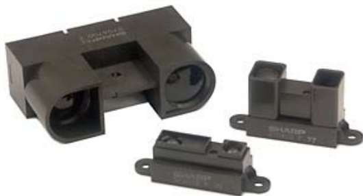
Figure 3. Sharp IR sensor variants and physical size [20].
