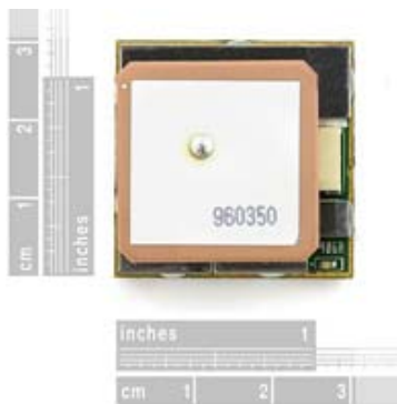
Figure 4. EM-406A GPS module from USGlobalSat [21]
