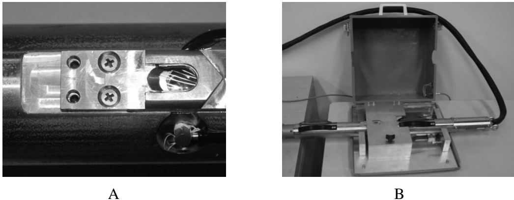
Figure 2 (A) X-ray window showing polypropylene and helium purge. (B) Bench top configuration.
