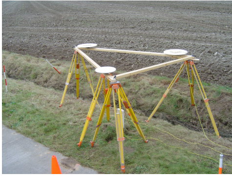
(a) Picture of the ground station set-up. (b) Scheme of the Ground Station set-up, reporting the two baselines lengths and the angle between them, as surveyed on field.
