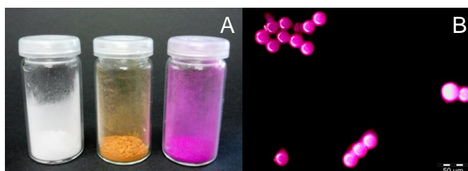
Figure 6. Optical photograph (A) of unmodified porous microspheres (left), microspheres after azide modification and click-attachment of NBD alkyne (middle), and alkyne-modified microspheres after click-attachment of Rhodamine B azide (right); dark field microscopy image (B) of Rhodamine B labelled microspheres MS6 (scale bar = 50 \mu\text{m} ).
