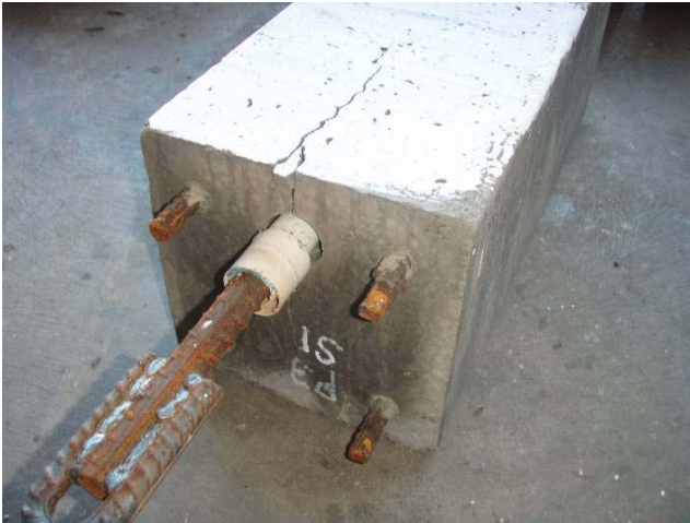
Fig. 3 (a) : Geopolymer concrete specimen
