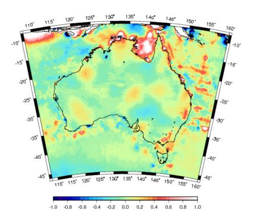
Figure 1: Differences (in metres) between EGM2008 and AUSGeoid98 (Lambert projection)
