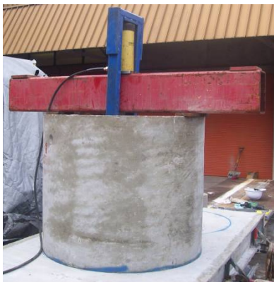
(a) Elevation showing spreader beam and jack
