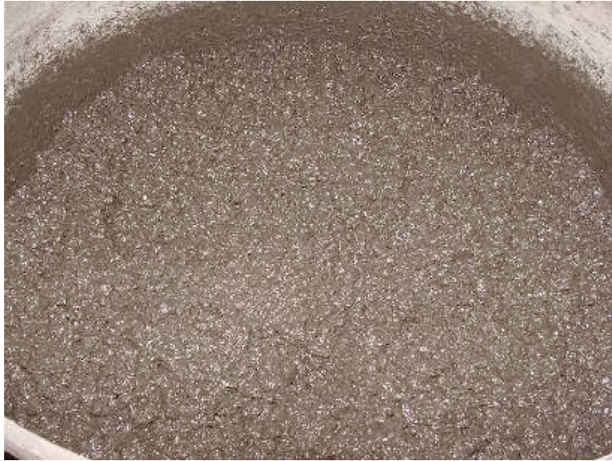
Figure 3.10: Fresh Geopolymer Concrete Ready for Placing
