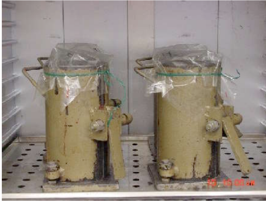
Figure 3.6: Wrapping Concrete Specimens Before Curing (2)
