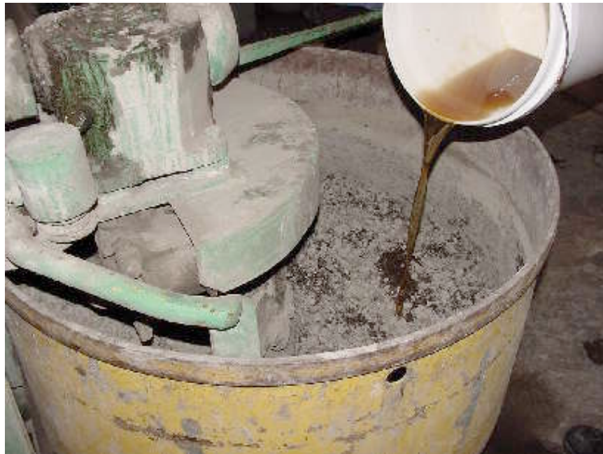
Figure 3.9: Addition of Liquid Component
