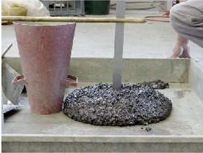
Figure 3.11: Slump Measurement of Fresh Concrete
