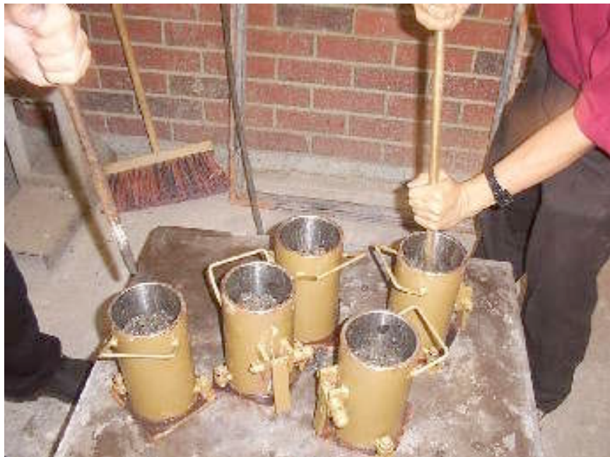
Figure 3.12: Compaction into Moulds
