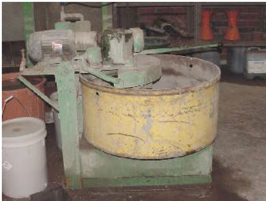
Figure 3.7: Pan Mixer Used for Manufacturing Geopolymer Concrete
