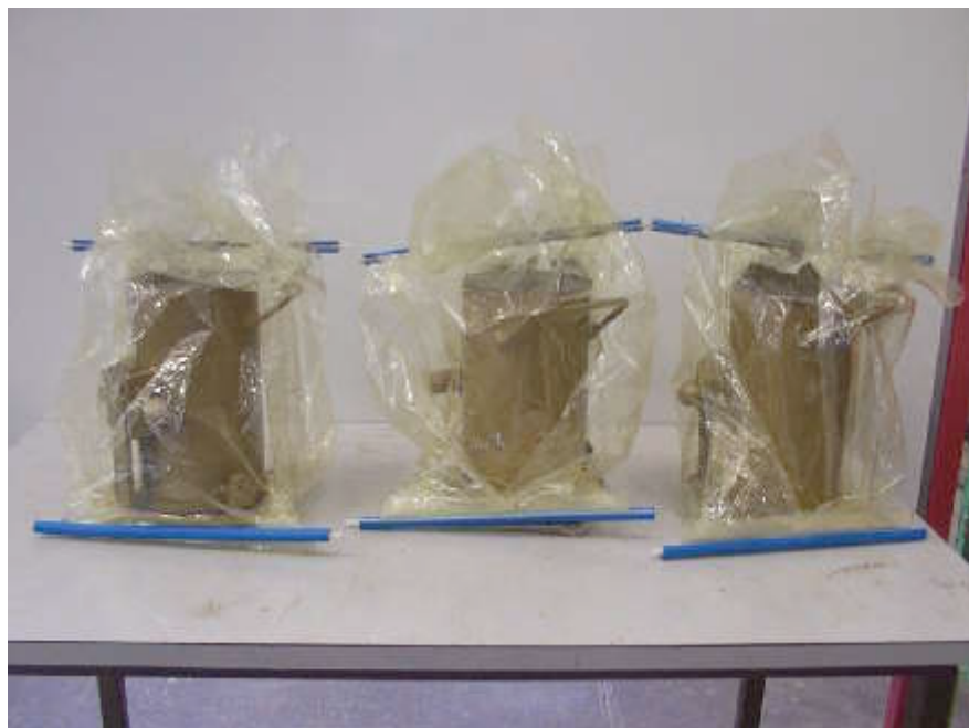
Figure 3.5: Wrapping of Concrete Specimens before Curing (1)
