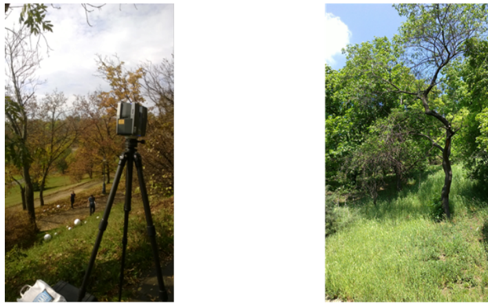
Figure 5: The test area covered by dense, but low vegetation. The left image indicates the tie points (i.e., reference points with known positions and radiuses) in white and the scanner while the right image shows the test area.
