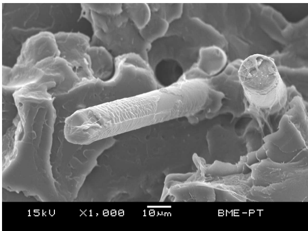
Fig.1. Cross-section of 20wt% basalt fiber reinforced PLA composite
