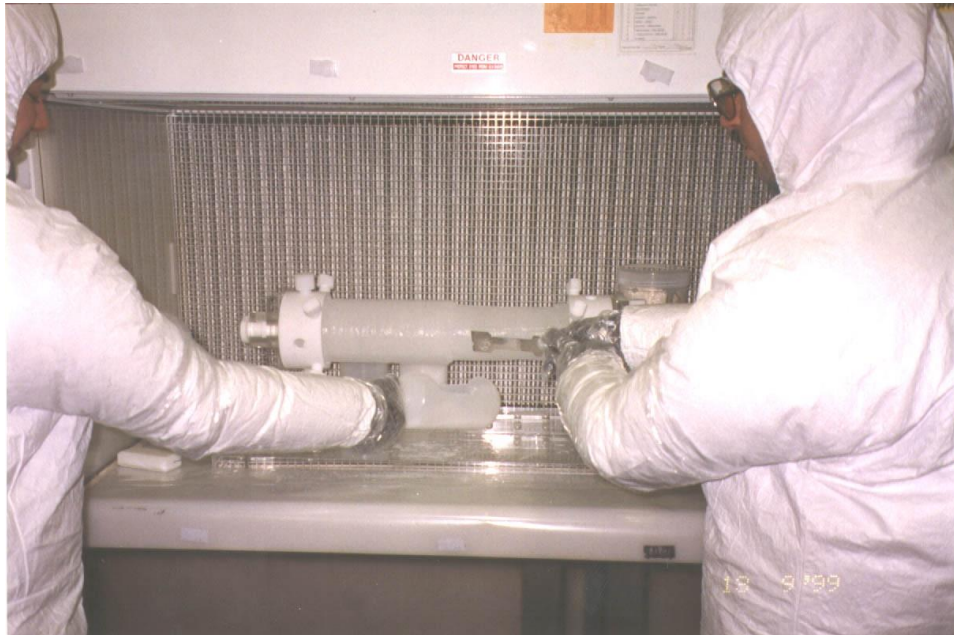
Figure 2.5. The decontamination technique used to remove the ice core veneers, with one operator chiselling the ice core, and the other collecting the chips in a plastic scoop. Photo by T. van Ommen.
