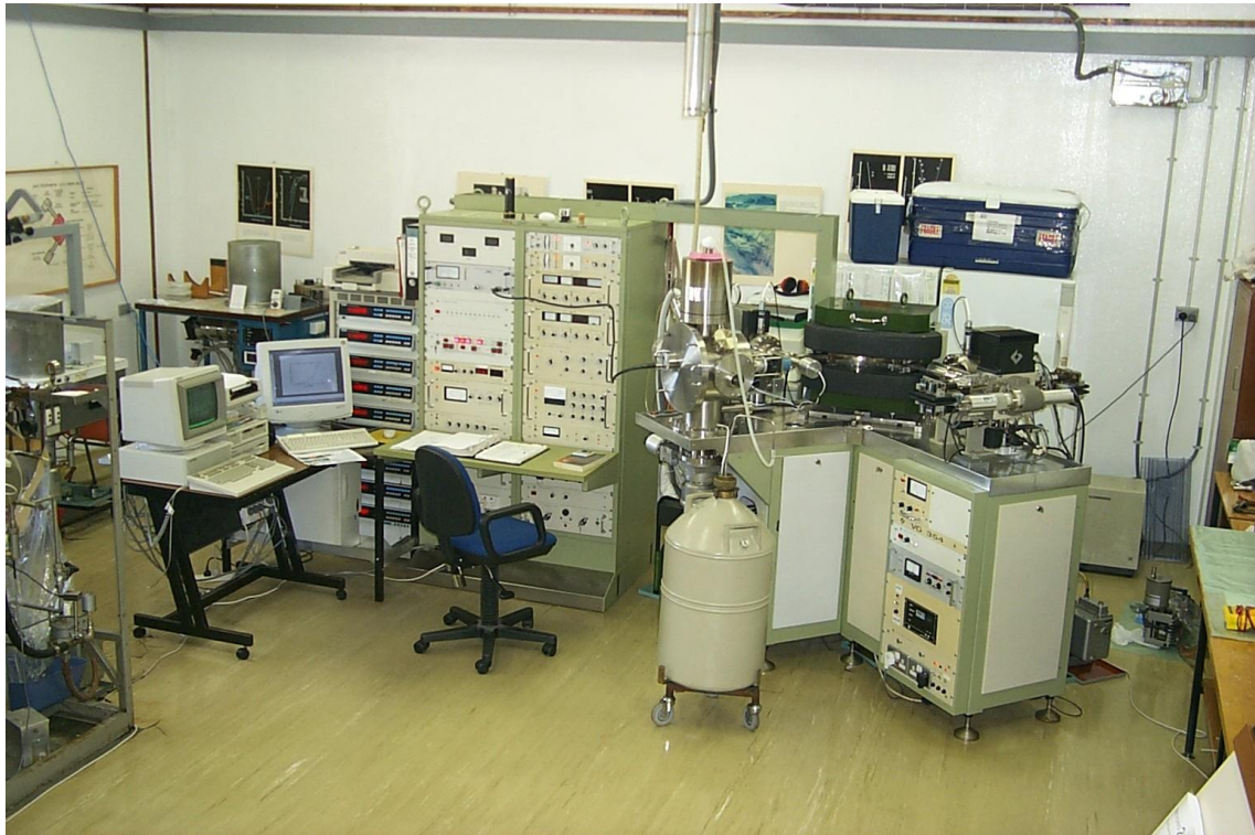
Figure 2.14 The VG 354 thermal ionisation mass spectrometer, operated within the School of Applied Physics at Curtin University. Photo by G. Burton.
