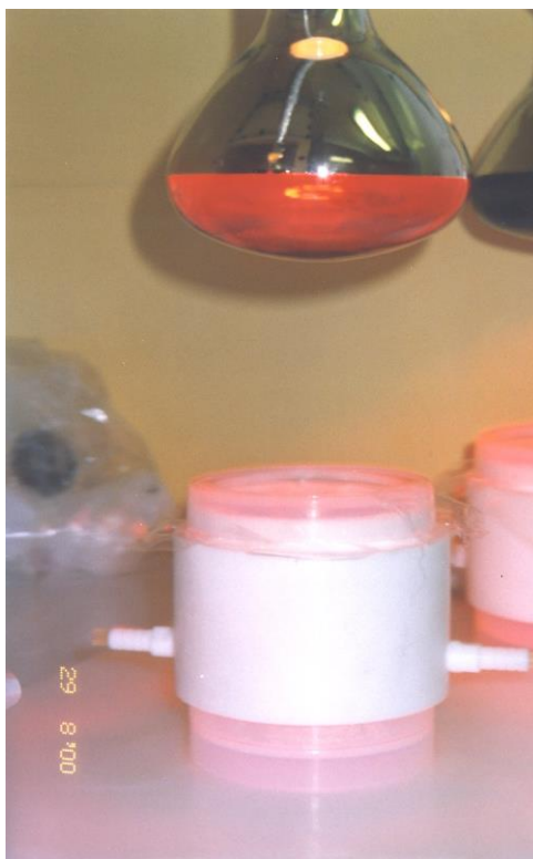
Figure 2.12. A Teflon™ chamber used for evaporating the samples, located under an infrared lamp. The beaker containing the sample is placed within the pot, on the Teflon PFA base, while the chamber is covered with clear Teflon FEP film. Photo by P. Vallelonga.
