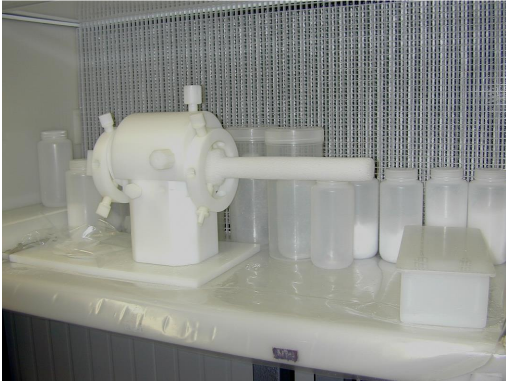
Figure 2.8. The new lathe designed for decontamination and high-resolution sampling of long ice cores. Photo by P. Vallelonga.
