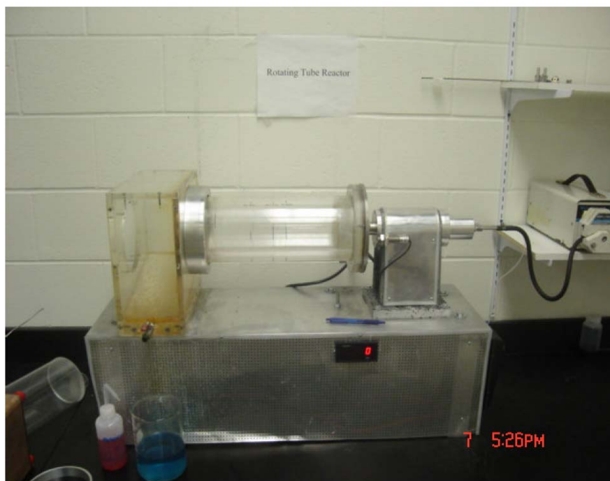
Figure 52 Image of the tube reactor [162]
