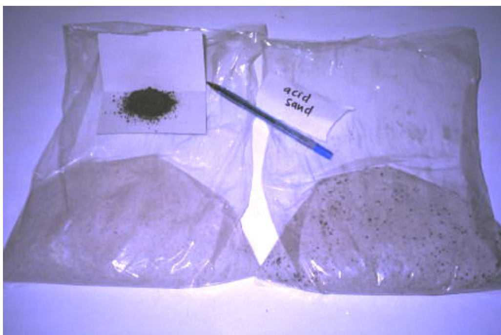
Plate 6.3 White (acid washed) sand before (left) and after (right) the addition of air-dried biosolids
