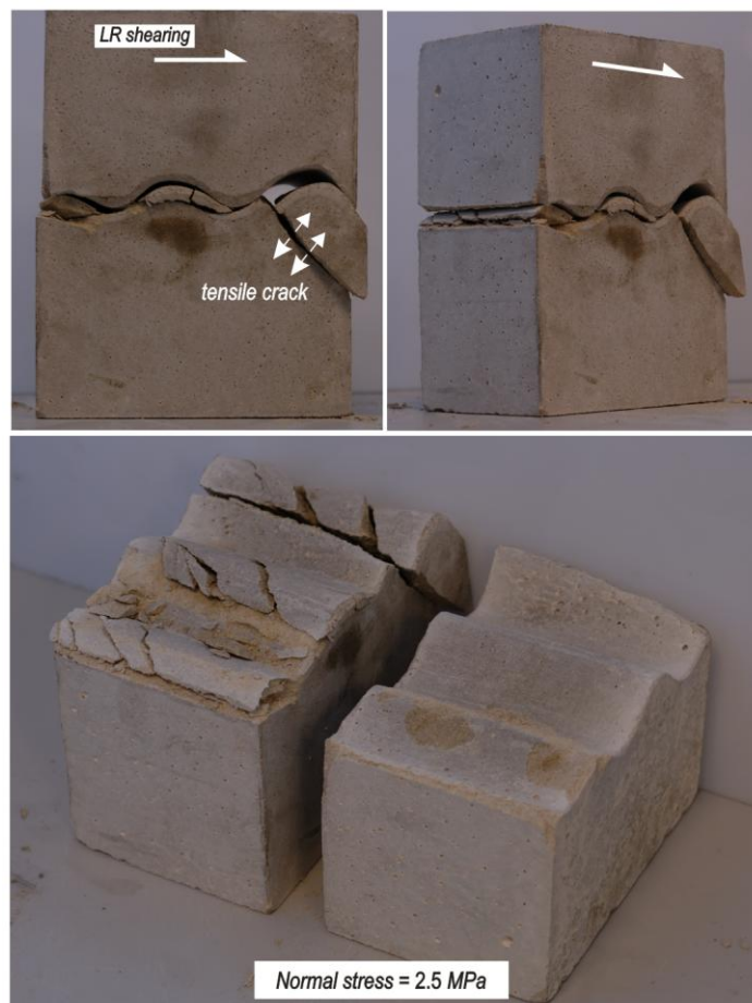
Figure 4.23 Profile B block view after shear tests under 2.5 MPa normal stress and 1.0 cm shear displacement from left to right.
