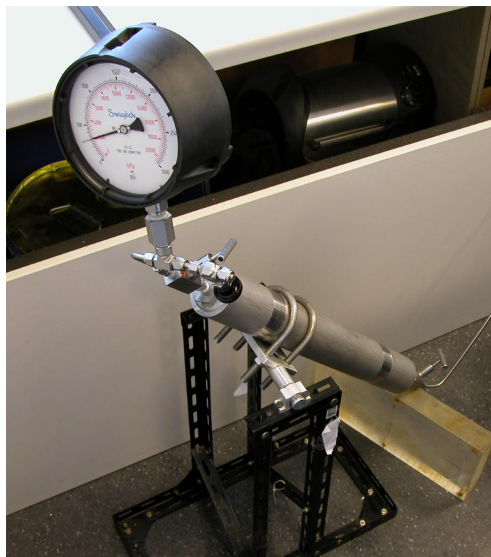
Figure 4.5 Duplex high pressure cylinder (DHPC) to apply constant normal load.
