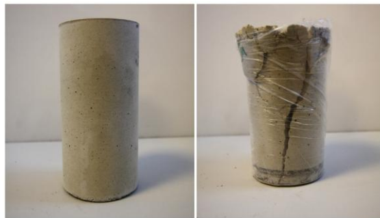
Figure 4.9 Cylindrical sample before and after the UCS test showing the shear failure plane.
