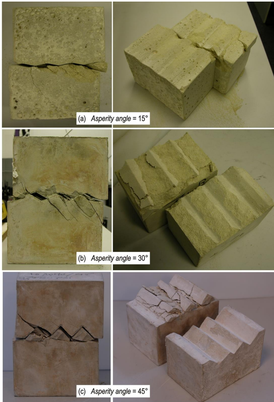
Figure 4.13 View of samples after shear experiments under 2.5 MPa normal stress.
