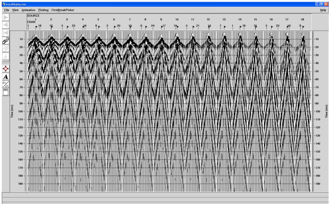
Figure 4.15: RVSP shot gathers obtained with seismic detonators as a seismic source for shots 1-18 (respectively from left to right) during the dry season.
