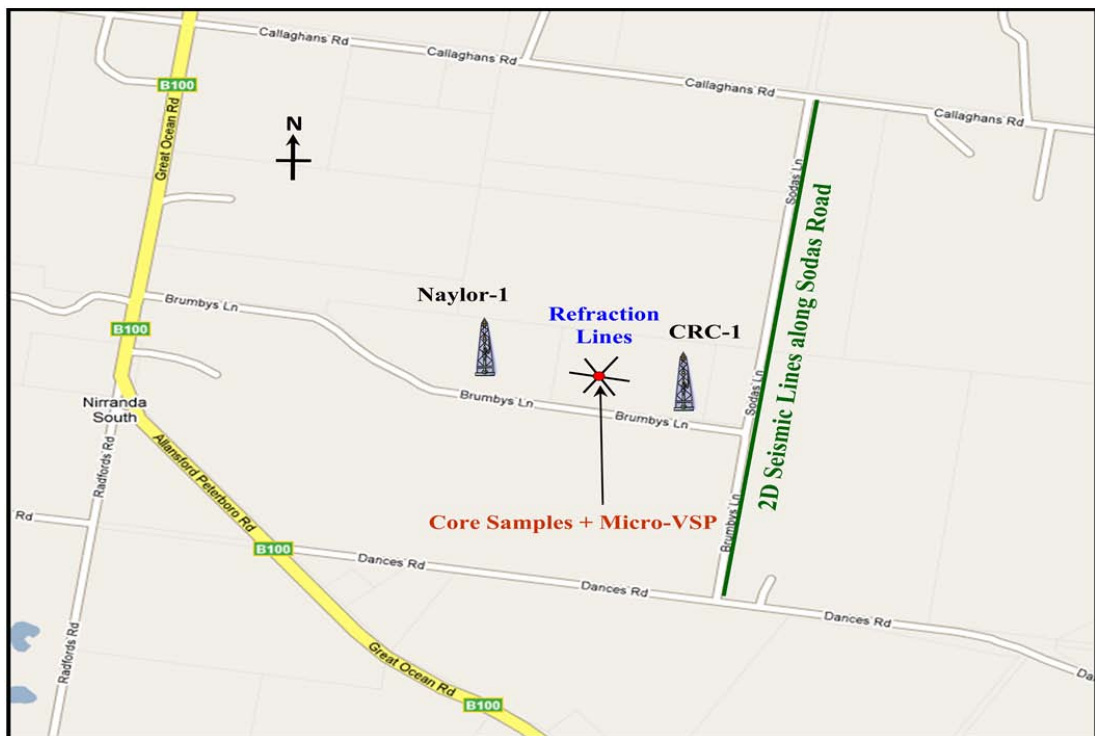
Figure 4.1: Location of the near-surface survey which has been acquired at the Naylor Field during both wet and dry conditions. The refraction surveys and micro-VSP data have been acquired in-between the Naylor-1 and CRC-1 wells, the distance between the Naylor-1 and CRC-1 wells is about 300m. The green line shows the location of the repeated 2D seismic test along Soda’s Road.
