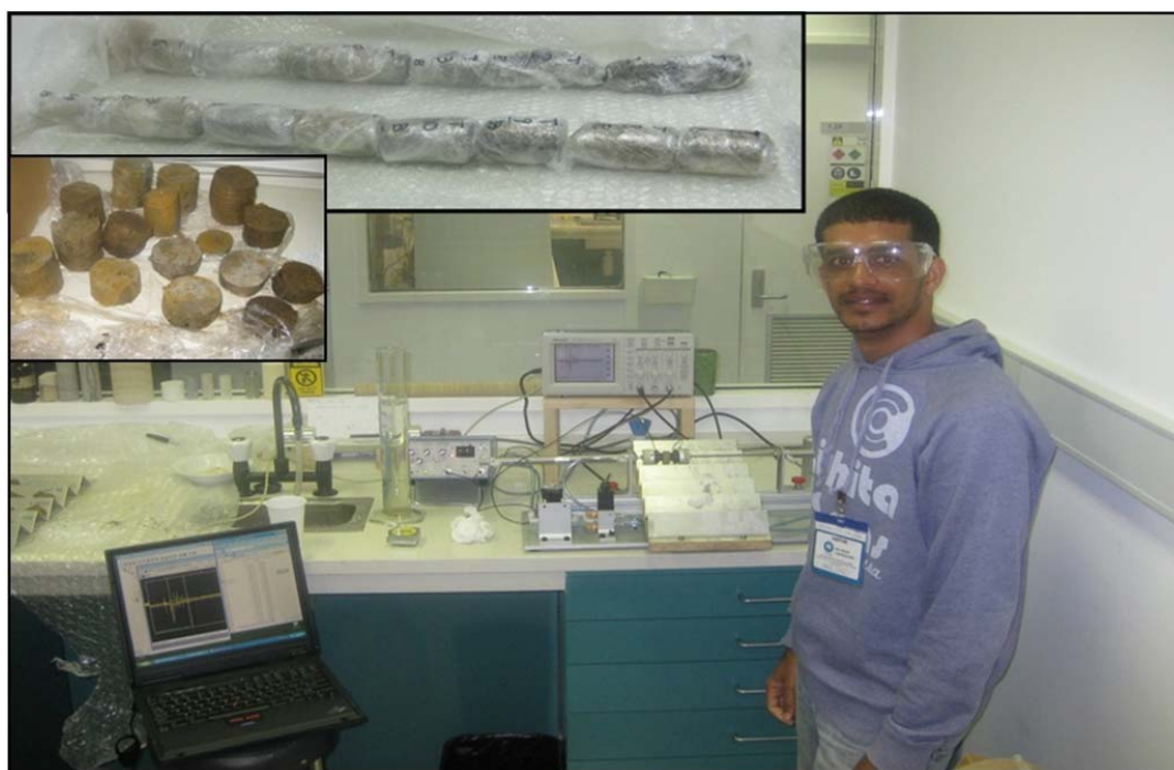
Figure 4.23: Ultrasonic measurements of the extracted core samples at the Ian Wark Laboratory, Petroleum Resources Department, CSIRO, Melbourne.
