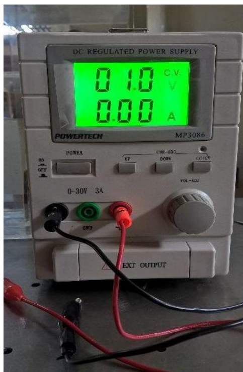
Figure 3-6. The DC supply power.
