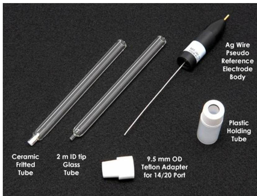
Figure 3-2. The constitution of the reference electrode.
