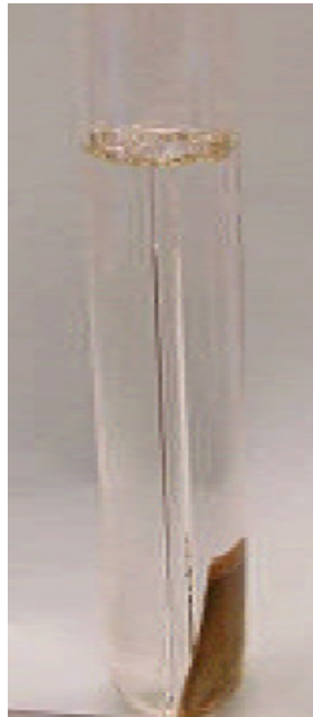
Figure 3-4 Test sample consist of copper strip wrapped with transformer paper impregnated in a 25g of new transformer oil.
