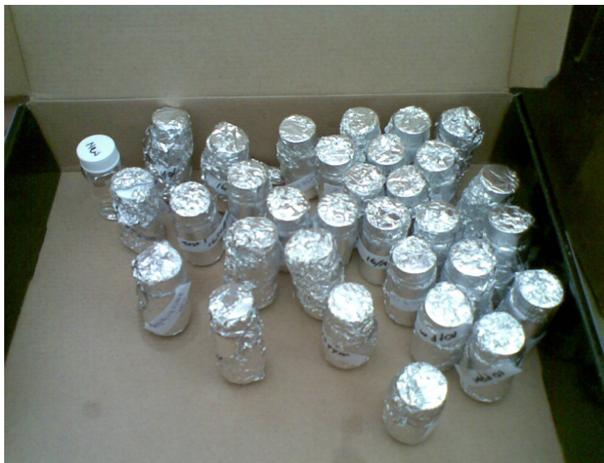
Figure 3-14: Sample collections of oil stored according to ASTM D923
