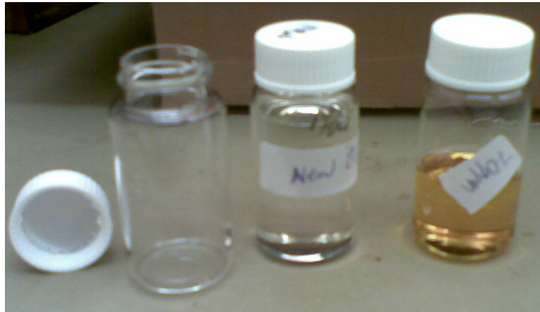
Figure 3-13 Sample collection of transformer oil with different furan content
