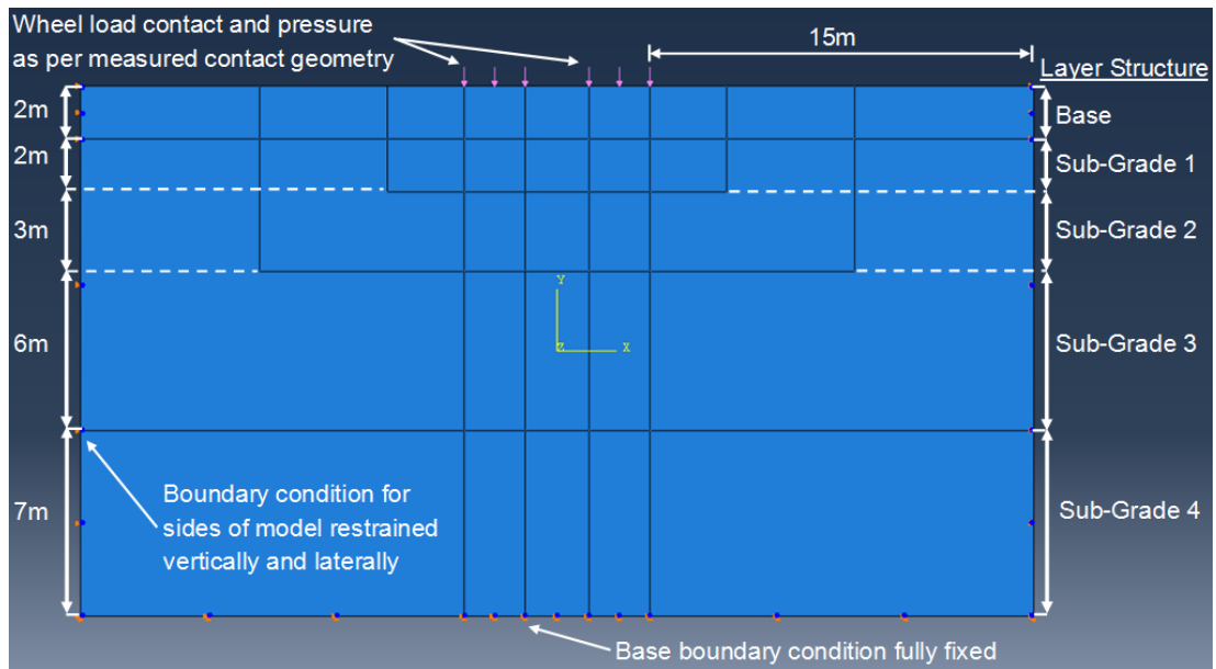
Figure 3.27: Annotated sketch of plane-strain FEA model.
