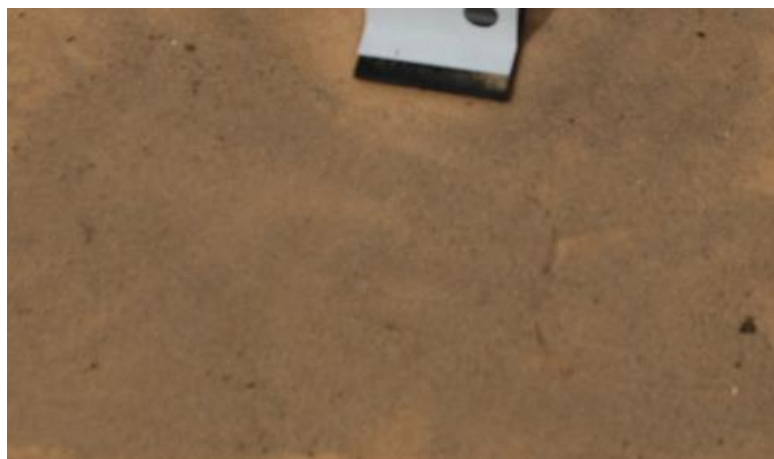
Figure B.2: Fine sand placed on test surface.
