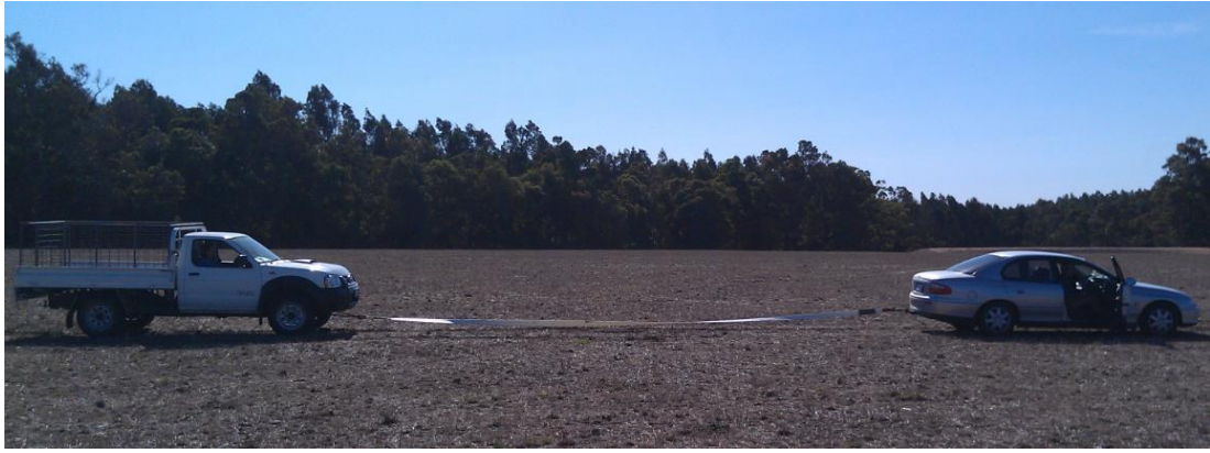
Figure 3.3: Photo of towed rolling resistance measurement trial test setup.
