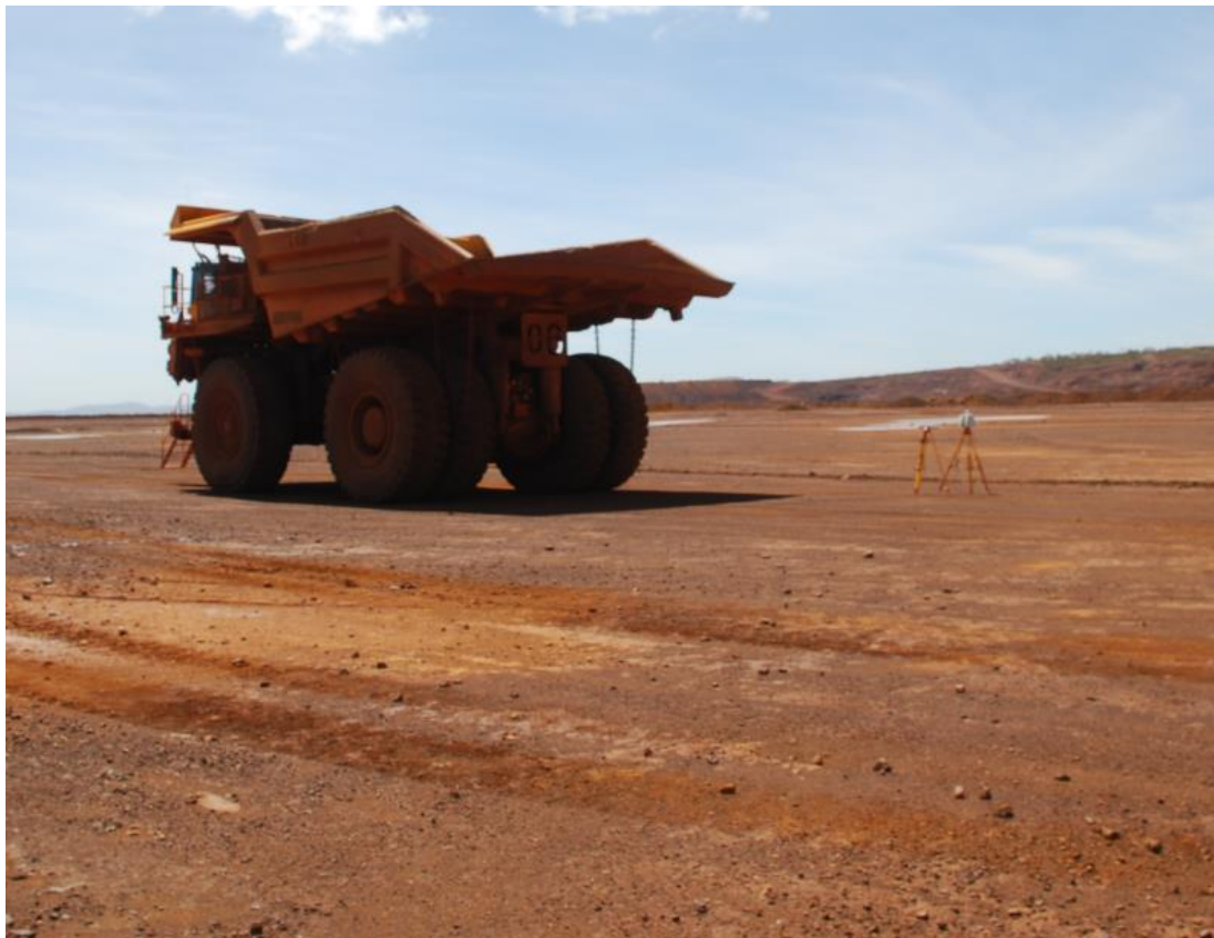
Figure 3.14: Setup of pavement deflection testing.
