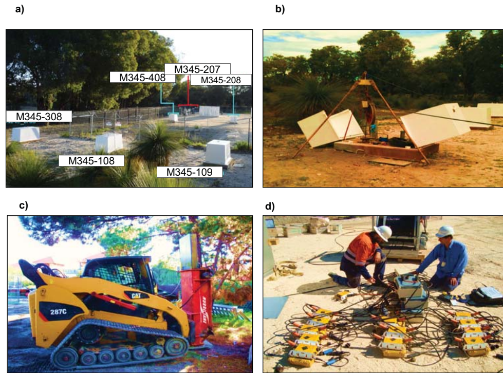
Figure 5-17. Field photographs for the equipment and site layout taken during acquisition. (a) The test site, which consists of one injection borehole (M345-207) and five monitoring boreholes (i.e., M345-208, -108, -109, -308 and -408) (modified from Malajczuk, 2010). (b) Hydrophone string deployed into the well M345-109. (c) 800 kg drop source. (d) Borehole acquisition system.
