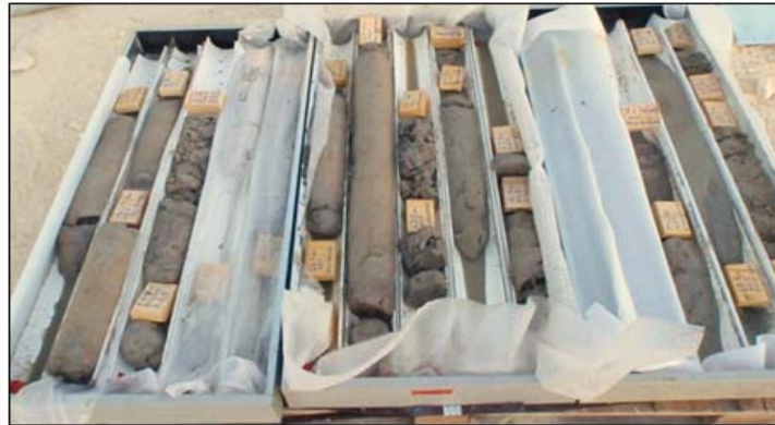
Figure 4-2. An example of core recovery and condition from drill hole NG3 from a depth of 50 to 70 m. These shallow sandstones are poorly-consolidated and core loss was common.
