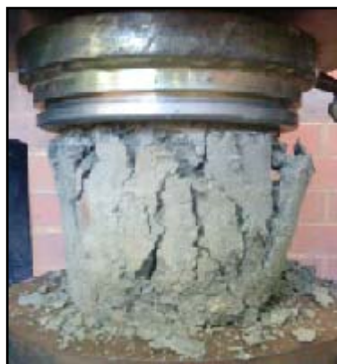
Figure 4: Unconfined Compressive Strength Test
