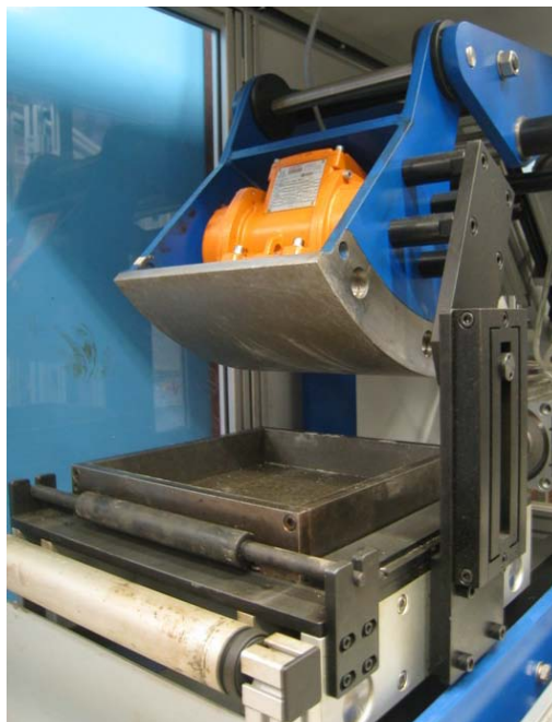
Figure 2. Cooper Compactor used to prepare slab specimens
