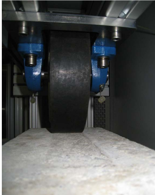
Figure 5. Typical Surface Depression After 5000 Runs
