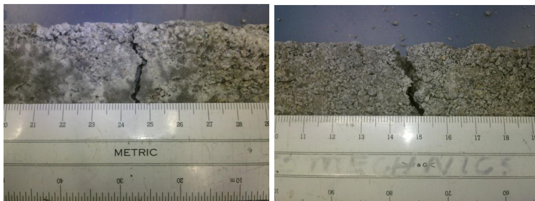
Figure 5.16: Location of failure plane along length of specimen
