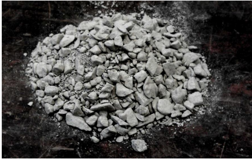
Figure 4.2: Crushed rock basecourse from Holcim Quarries Pty Ltd
