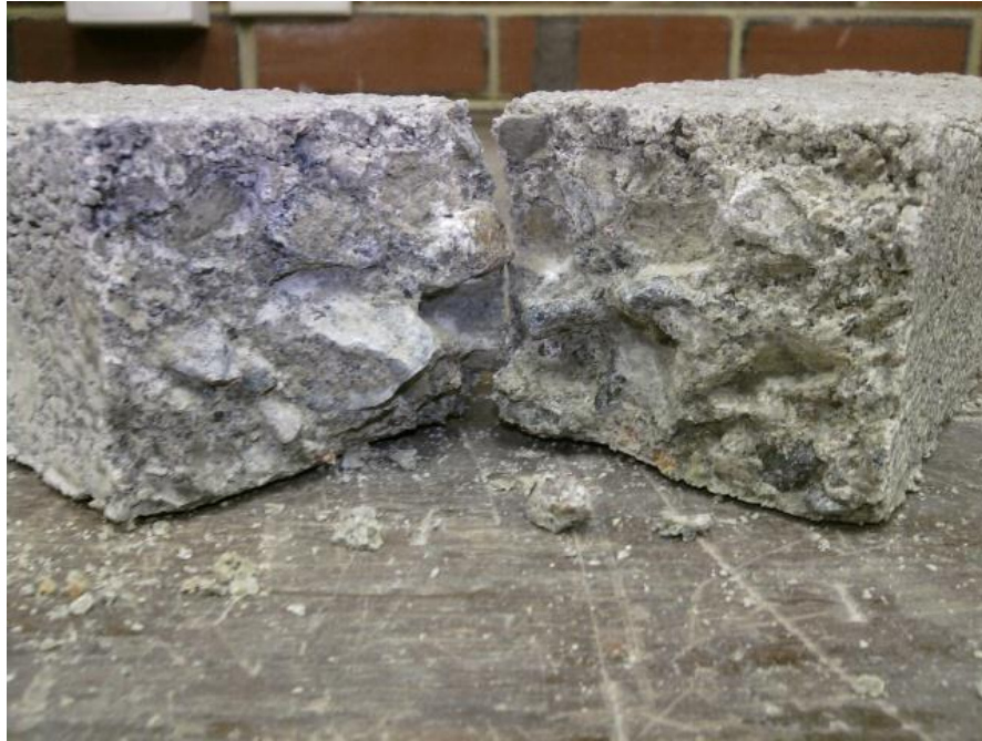
Figure 5.17: Failure section of flexural beam specimen after fatigue loading
