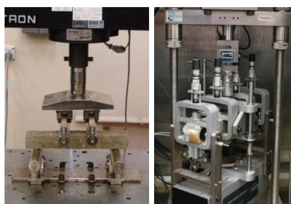
Figure 2: Four Point Bending Test Setup – Static and Dynamic
