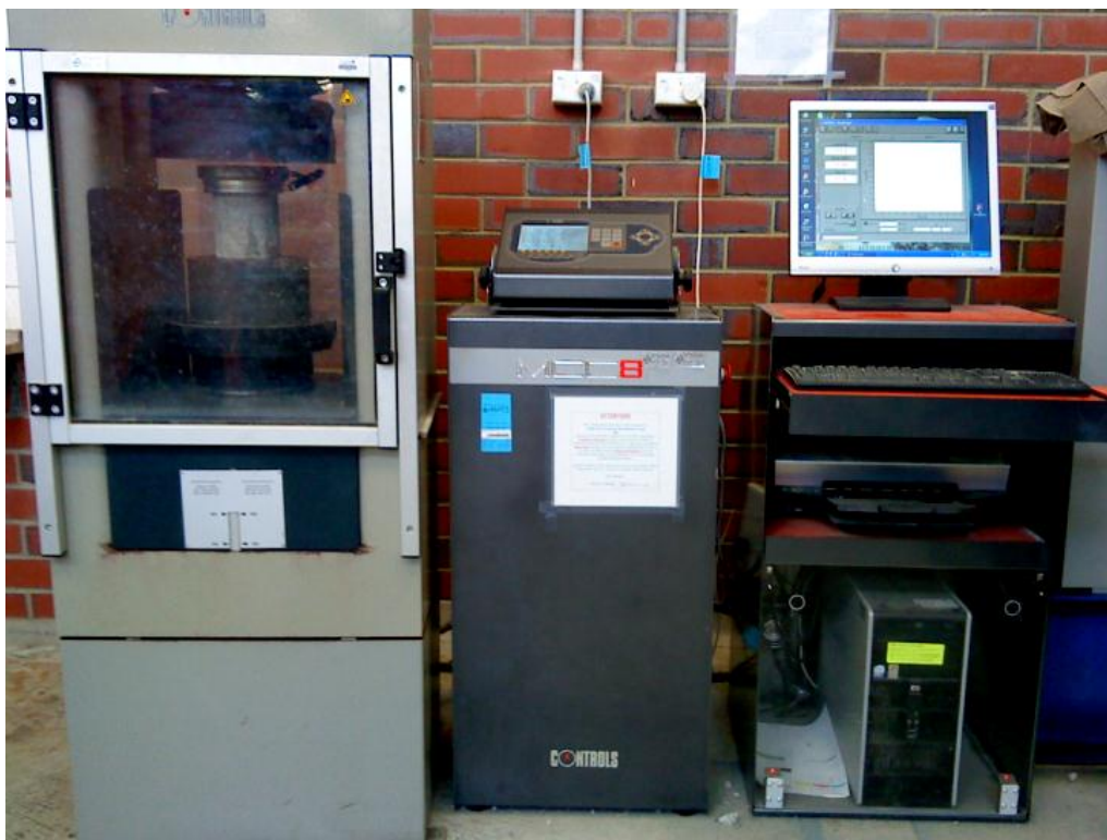
Figure 4.3: Controls MCC 8 Computerised Control Console for UCS tests
