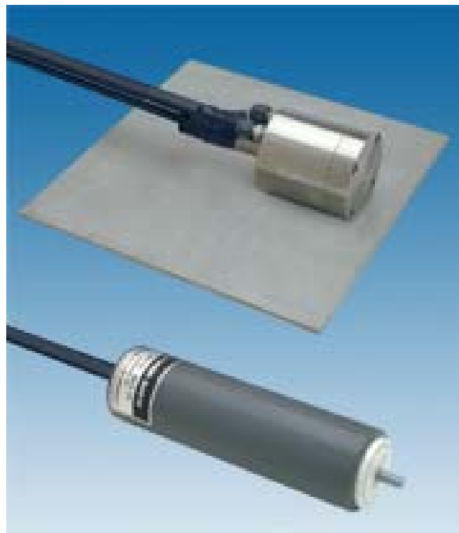
Figure 7.15 Liquid settlement gauge (Courtesy of Sinco).
