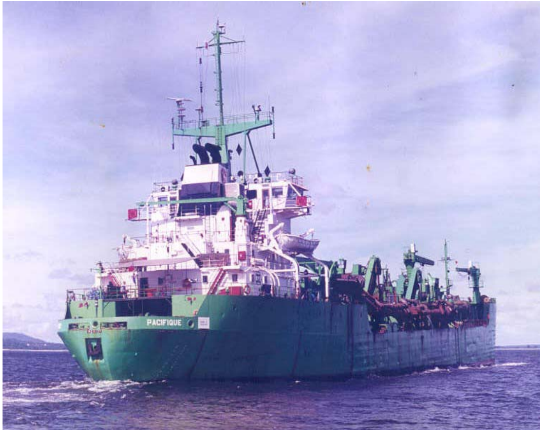
Figure 4.7 Trailer suction hopper dredger in operation.
