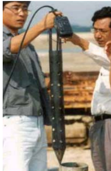
Figure 7.17 Typical details and photo of pneumatic piezometer with protected guard cell. (photo courtesy of Dr M.W.Bo).
