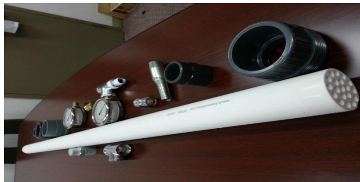
Ceramic membrane, pressure gauges and connectors
