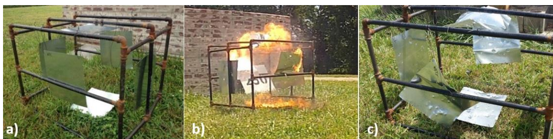
Figure 5.6: Photographs of the PVC pipe bomb trial set-up, a) prior to; b) during; and c) following initiation of the device.
