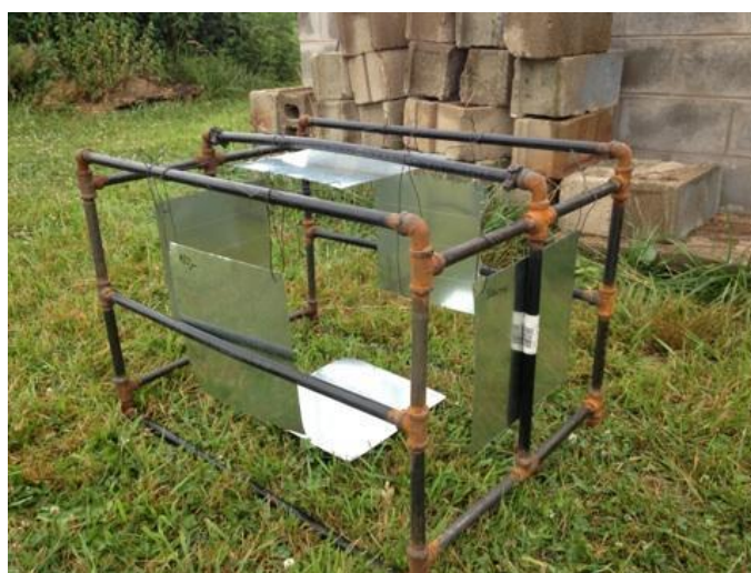
Figure 5.1: Pipe bomb detonation trial set-up showing galvanised steel witness plates attached to each side of the welded metal frame surrounding the device.
