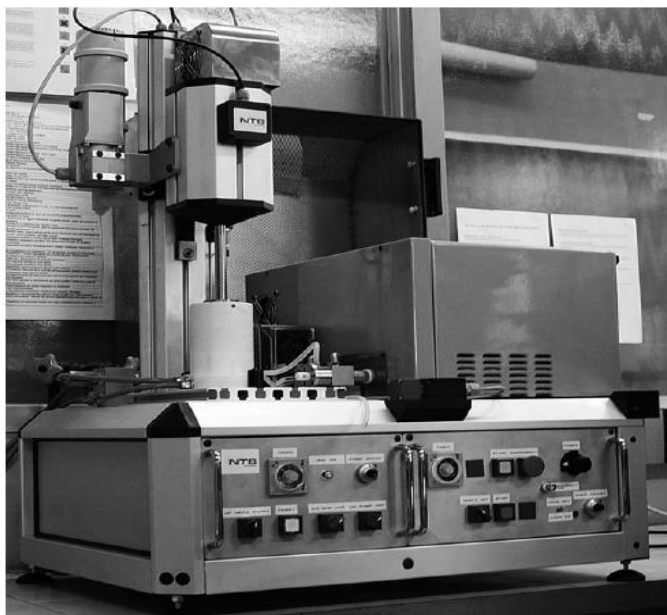
Figure 2.10 Overall picture of a flow reactor combining MW and US irradiation in a sequential mode (Cravotto and Cintas, 2007).
