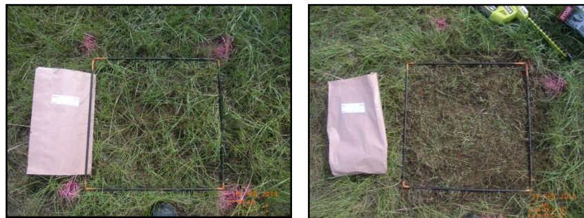
Figure 3.1: A field AGB 50 × 50 cm quadrat before (left) and after harvesting a cut sample (right).
