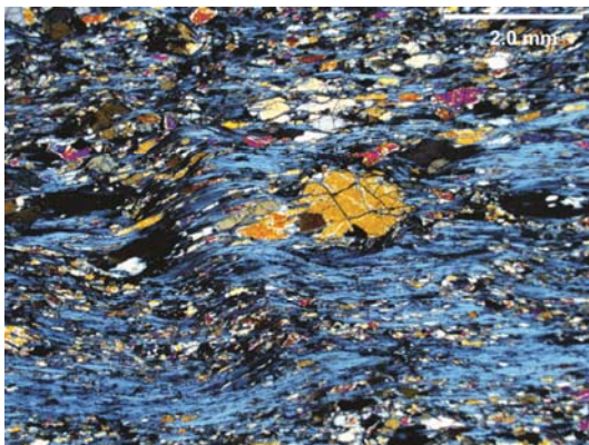
Porphyroclastic olivine in a pervasively foliated matrix of antigorite and neoblastic olivine.
