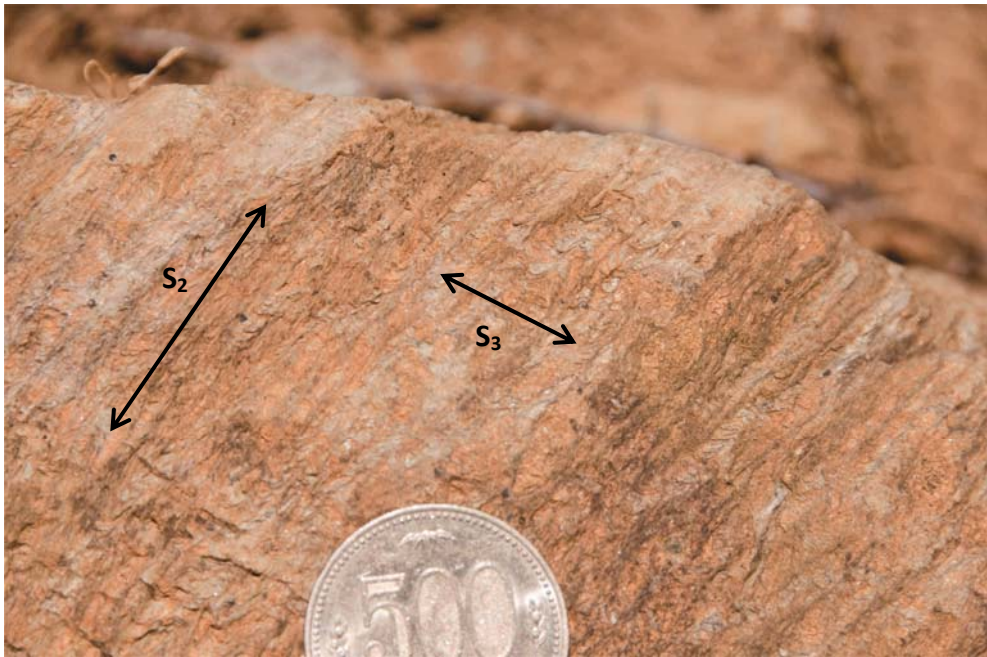
Figure 3.16. Multiple generations of foliation development in a dunite from Mt. Higashi-Akaishi. S_2 is generally defined by the alignment of olivine, chromite and antigorite. S_3 crenulates S_2 and is generally defined by antigorite alignment.
