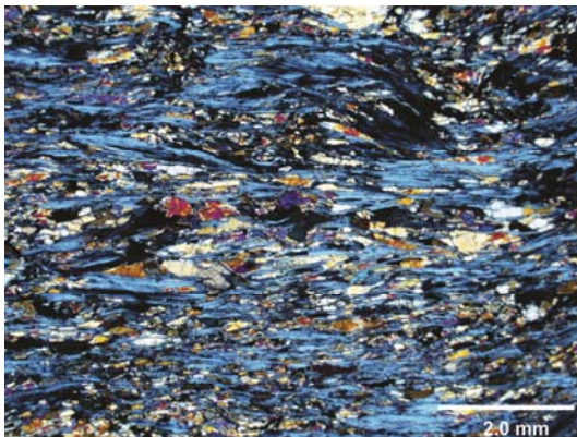
XPL image of the antigorite-rich microlithon showing extensive antigorite growth and alignment parallel to the lineation direction (E-W).
