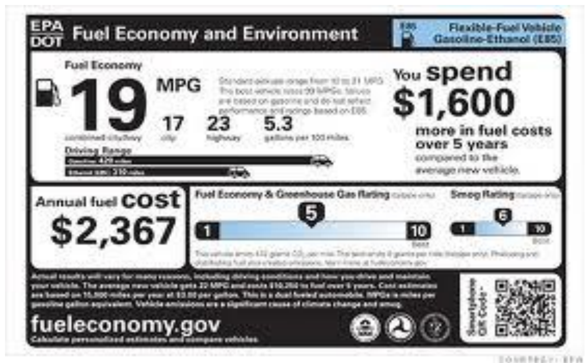
FIGURE 4.2: The US Fuel Economy and Environment Label for a Gasoline Vehicle with Gas Guzzler Tax
