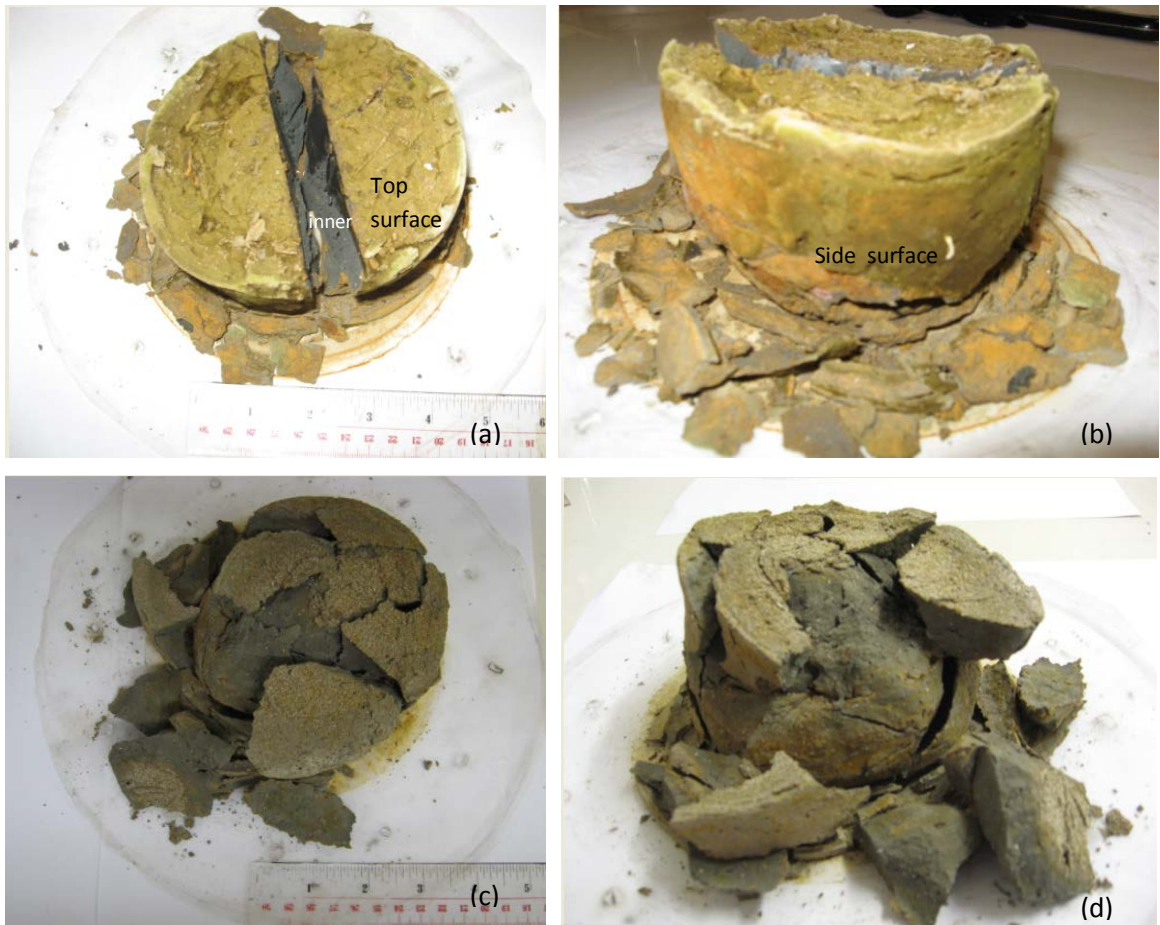
Figure 4.2: Residual material after 12 weeks' oxidation (a) the material from group 1 (weekly drying), displaying top surface; (b) the material from group 1, displaying side surface and bottom surface; (c) the material from group 2 (monthly drying); (d) the material from group 3 (three month drying). The images show visual oxidation signs of yellow-brown on the top and side surface with gley colours in the inner part.
