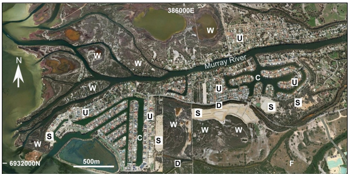
Figure 3.5: Aerial image of the South Yunderup area showing the main landforms – wetlands (W), drains (D), exposed floodplains (F), compacted dredged material flats (S), canals (C) and urban construction and townships (U). Modified from Google earth.
