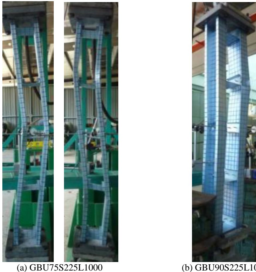
Figure 4.43: Failure Modes of Tested S225L1000 Built-up Columns with a Gap
