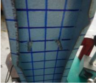
Figure 4.36: Failure Modes at Mid-Length of Tested BU75L1000 Built-up Columns
