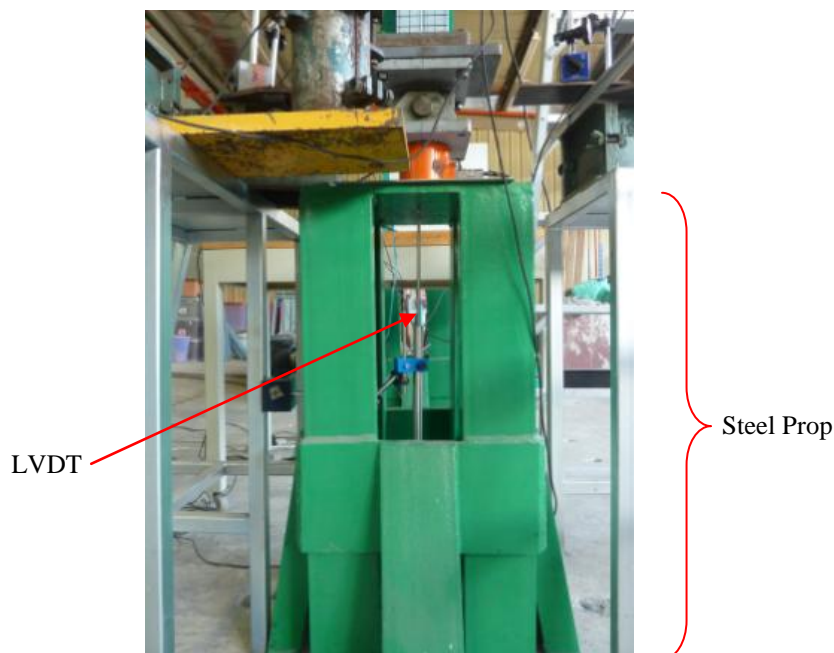
Figure 4.11: LVDT measuring plate deflection
