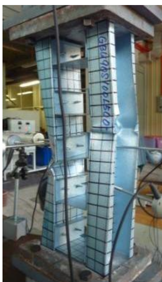
Figure 4.6: GBU90S100L500-4 Failed with a Mixed Failure in x and y-axis
