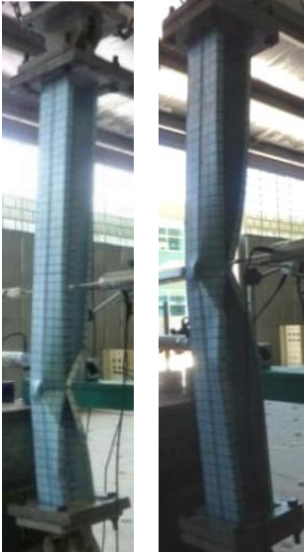
Figure 4.34: Failure Modes of Tested BU90S225L1000 Built-up Columns
