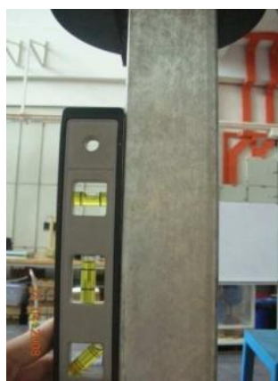
(b) Level used to examine straightness of the specimens
