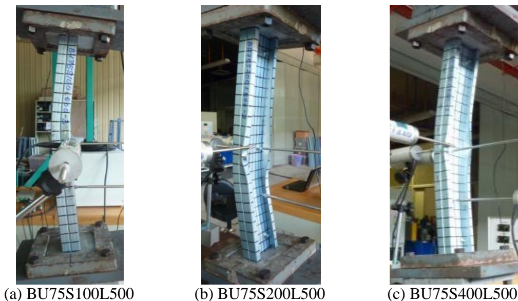
Figure 4.32: Failure of Tested BU75L500 Built-up Columns
