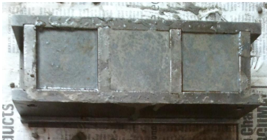
Figure 3.17: Mortar Test Cubes
