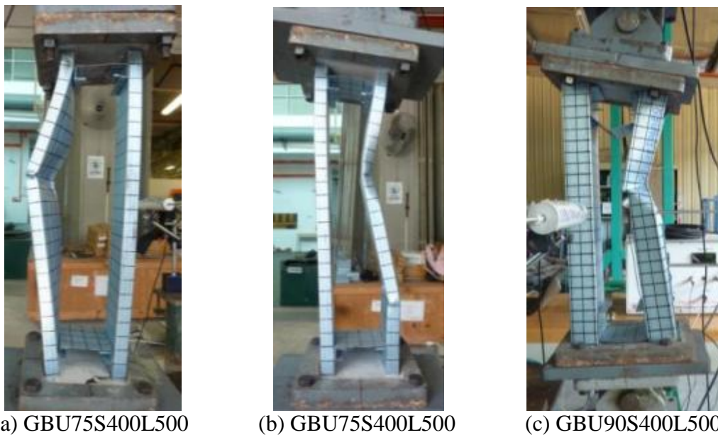
Figure 4.42: Failure Modes of Tested S400L500 Built-up Columns with a Gap
