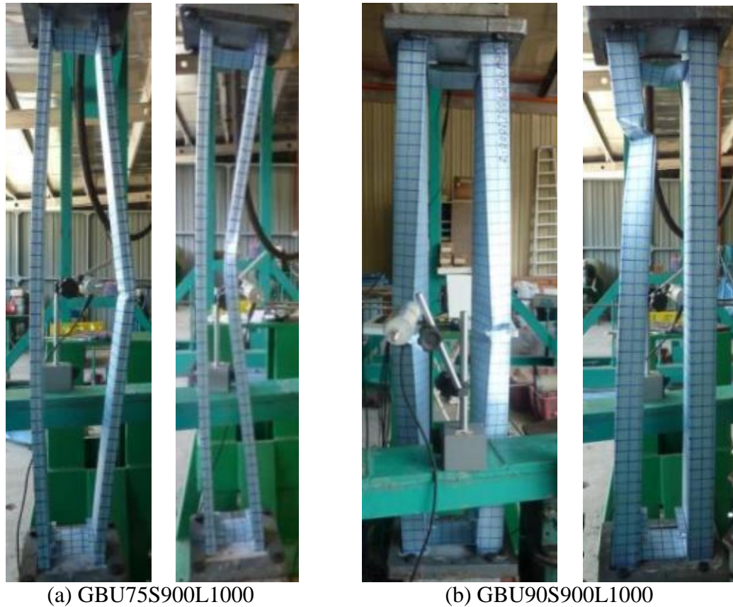
Figure 4.44: Failure Modes of Tested S900L1000 Built-up Columns with a Gap
