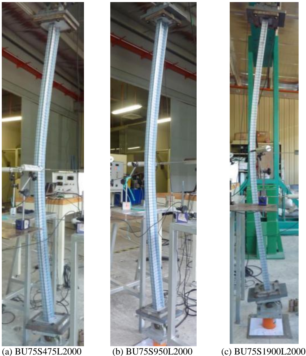
Figure 4.38: Failure Modes of Tested BU75L2000 Built-up Columns
