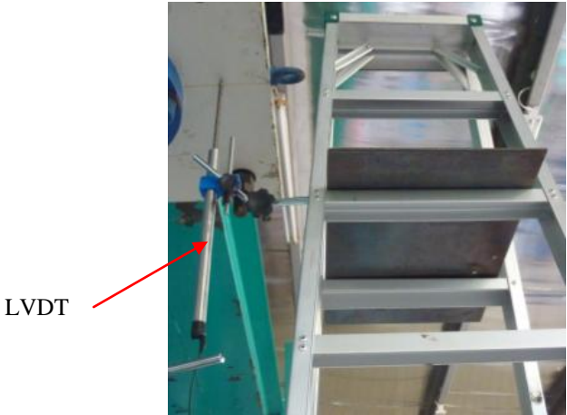
Figure 4.10: LVDT measuring beam deflection
