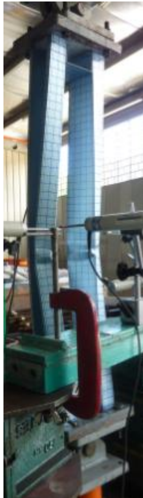
Figure 4.8: Failure modes of GBU90S900L1000-2
