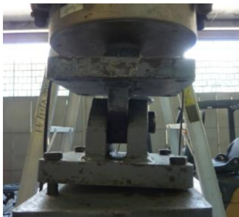
Figure 4.3: Failure of Pinned-end when Testing BU90S225L1000-3
