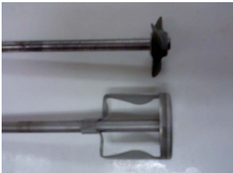
Figure 2.31: The two types of impellers used in these experiments. Standard impeller is at the top, Aldrich Z17143-3 at the bottom.
