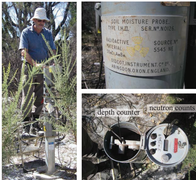
Figure 6.7: Neutron logging in the field with Didcot Neutron moisture probe.
