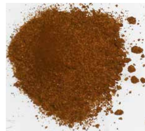
Figure 3.14: Pictures of samples collected on the Gngangara Mound for dielectric lab measurements. Note that the cemented "coffee rock" material and Mandalay Beach ferricrete were broken up in order to fill the dielectric cell.
