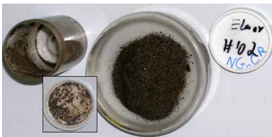
Figure 3.14: Pictures of samples collected on the Gngangara Mound for dielectric lab measurements. Note that the cemented "coffee rock" material and Mandalay Beach ferricrete were broken up in order to fill the dielectric cell.
