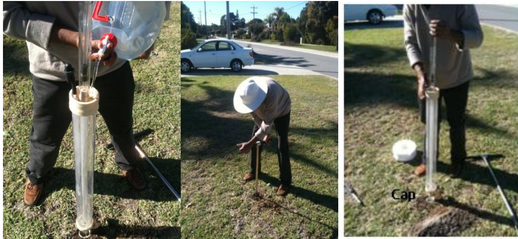
Figure 23. Field testing procedure using Guelph Permeameter
