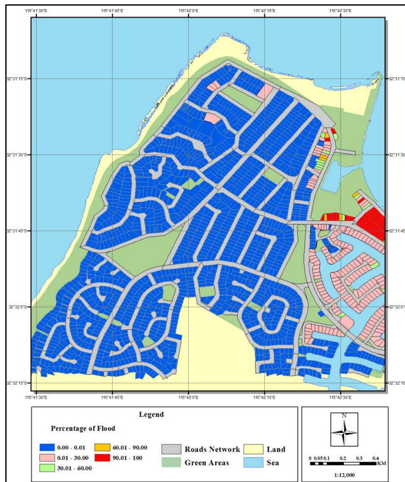
Figure 5.12 Property-based percentage of flooding for the Mandurah study area, assuming a sea level rise of 2.06 m.
