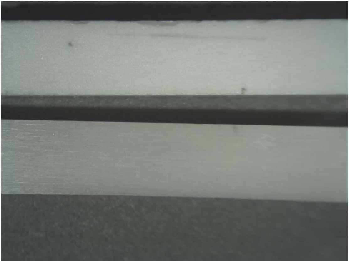
Figure S 7 Optical Micrograph of 2 MOR bars showing difference in optical properties
